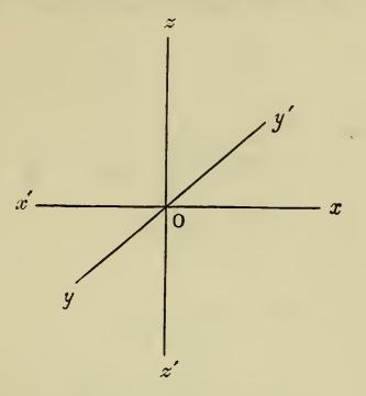
nates of a point whose absolute distances from the co-ordinate planes are  $\alpha$ ,  $\beta$ ,  $\gamma$  are represented by  $(\alpha, \beta, \gamma)$ ,  $(-\alpha, \beta, \gamma)$ ,  $(\alpha, -\beta, \gamma)$ ,  $(\alpha, \beta, -\gamma)$ ,  $(\alpha, -\beta, -\gamma)$ ,  $(-\alpha, \beta, -\gamma)$ ,  $(-\alpha, -\beta, \gamma)$ ,  $(-\alpha, -\beta, -\gamma)$ , according as the point lies in the compartment Oxyz, Ox'yz, Oxy'z, Oxyz', Oxy'z', Ox'yz', Ox'y'z, Ox'y'z', respectively.
